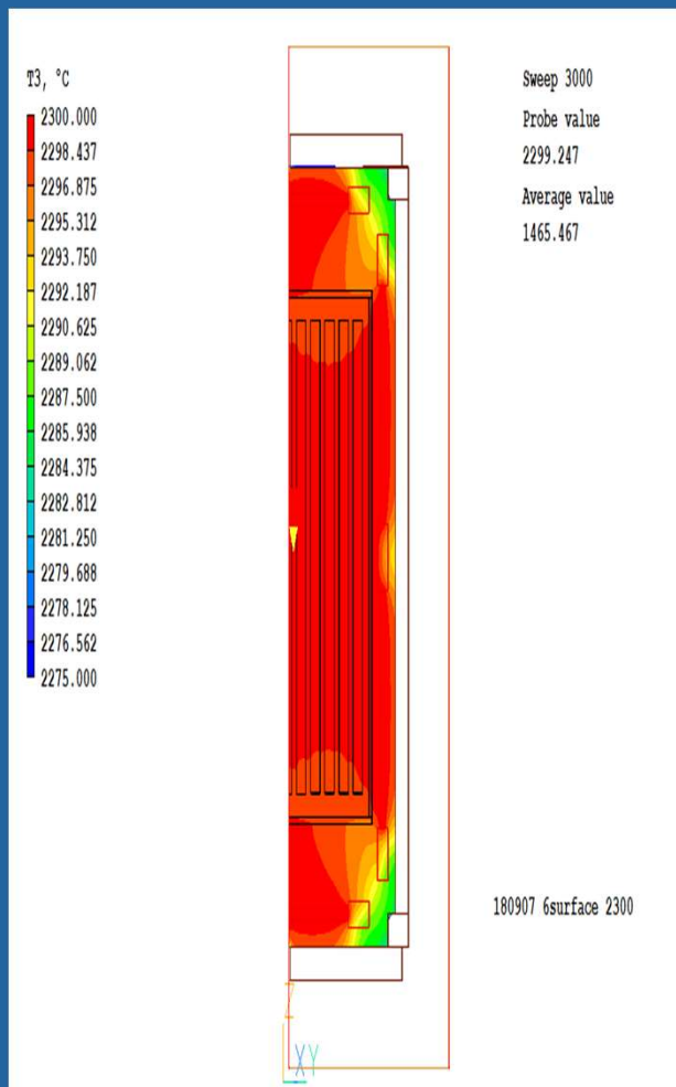
▲ Uniformity of 6 side heating
